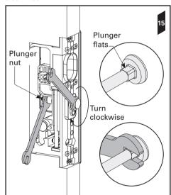
**16.** Continue to turn the spanner until there is no longer a gap between the spanner and the chassis.
