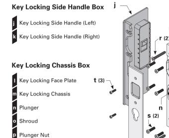
Note: Components will vary between the 'Key One Side', 'Key/Key' and 'Key/Snib' versions.
