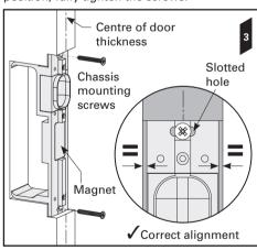
4. Fit the 6x side handle to chassis screws. eave a 3mm gap (1/8") between the underside of the screw head and the chassis.
